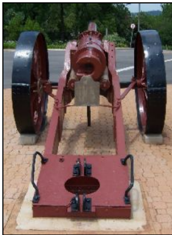
The gun's breech. Note the firing block was removed, presumably by the Germans when they abandoned it, so that it didn't fall into allied hands while in working order.
