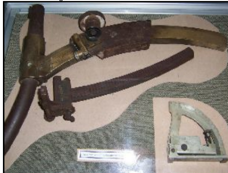
A sight arc from one of the Königsberg 10.5cm guns on display at the South African National Museum of Military History.
