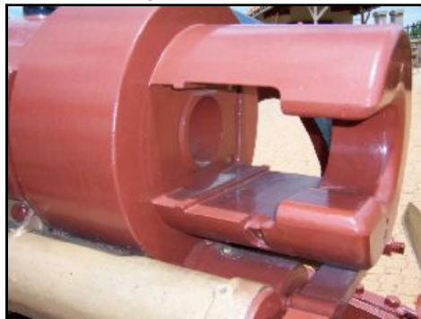
The gun's breech. Note the firing block was removed, presumably by the Germans when they abandoned it, so that it didn't fall into allied hands while in working order.
