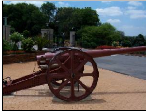
...and after restoration. Note its "new" colour, a reddish brown. During restoration paint samples were taken and it was found this was the colour of the gun as seen during the First World War. The gun was mounted on its chassis at Dar-es-Salaam railway works so presumably this was the colour used on trains in German East Africa at the time.
