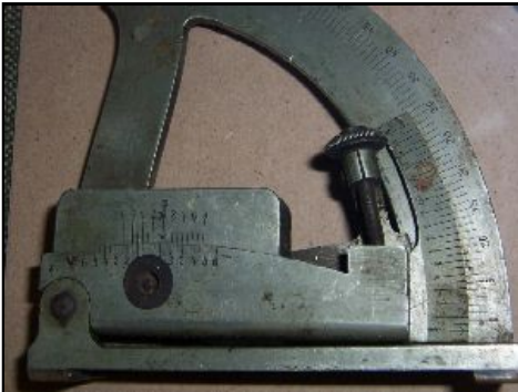
A quadrant used with a 10.5cm Königsberg gun on display at the South African National Museum of Military History
