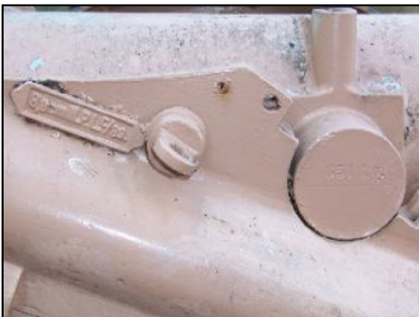
Markings on the right side of the gun. They read "8.8cm", the calibre of the gun "M.P.L.c/89" for Mittel-Pivot-Lafette" or Central Pivot Carriage model of 1889, and further down is the weight of the gun "651kg".
